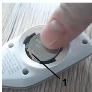
Slide the battery under the golden metal tab (1). Make sure that the battery is completely under the metal nose and pushed completely to the upper edge. Push the battery into the socket by pressing lightly on the opposite side until you hear a short "click".
