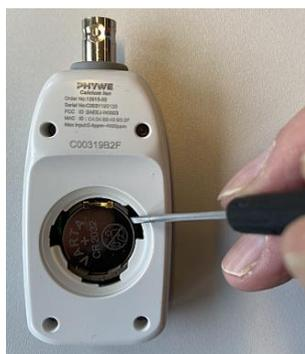
Lever the battery sensitively, e.g. with the help of a small screwdriver, or small scissors from the socket. Place the screwdriver like this, as can be seen in the illustration.
