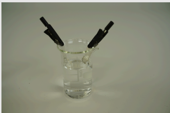
Attachment of the electrode plates to the rim of the beaker.
