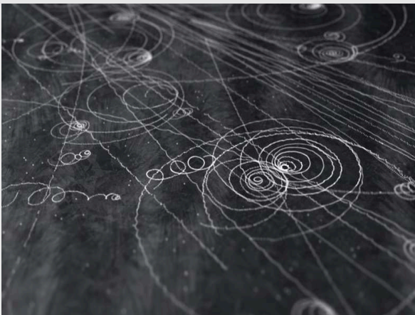
Particle tracks detected in a cloud chamber show curved paths for some particles
