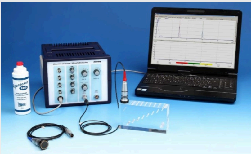
Fig. 1: Equipment for ultrasonic echography, experimental set-up
