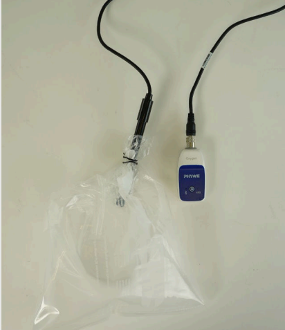
Setup for collecting the breathing air
