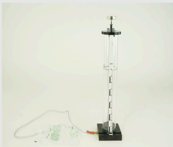
Setup of the gasometer
