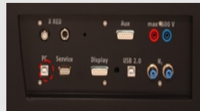
Fig. 5: Connection of the computer
