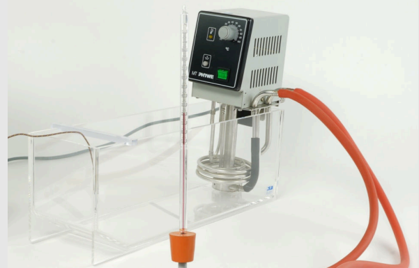
Fig.3. Experimental set-up for measuring thermal expansion
