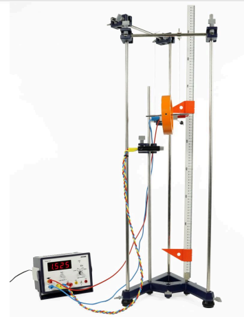
Fig. 2: Experimental set-up for investigating the conservation of energy, using the Maxwell disk.
