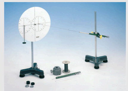
Fig.1: Experimental set-up for investigating moments in equilibrium.
