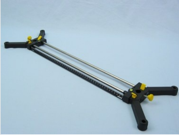
Assembly of the optical bench
