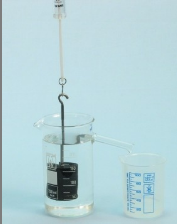
Determination of the weight forces in water
