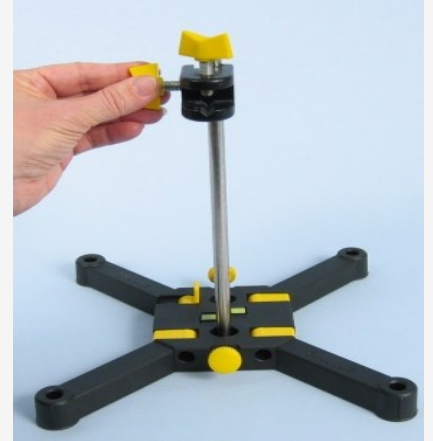
Attaching the double socket to the stand rod
