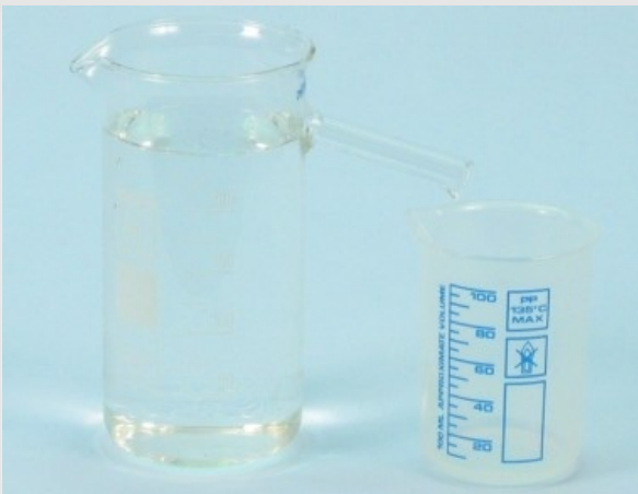
Filling the overflow vessel with water
