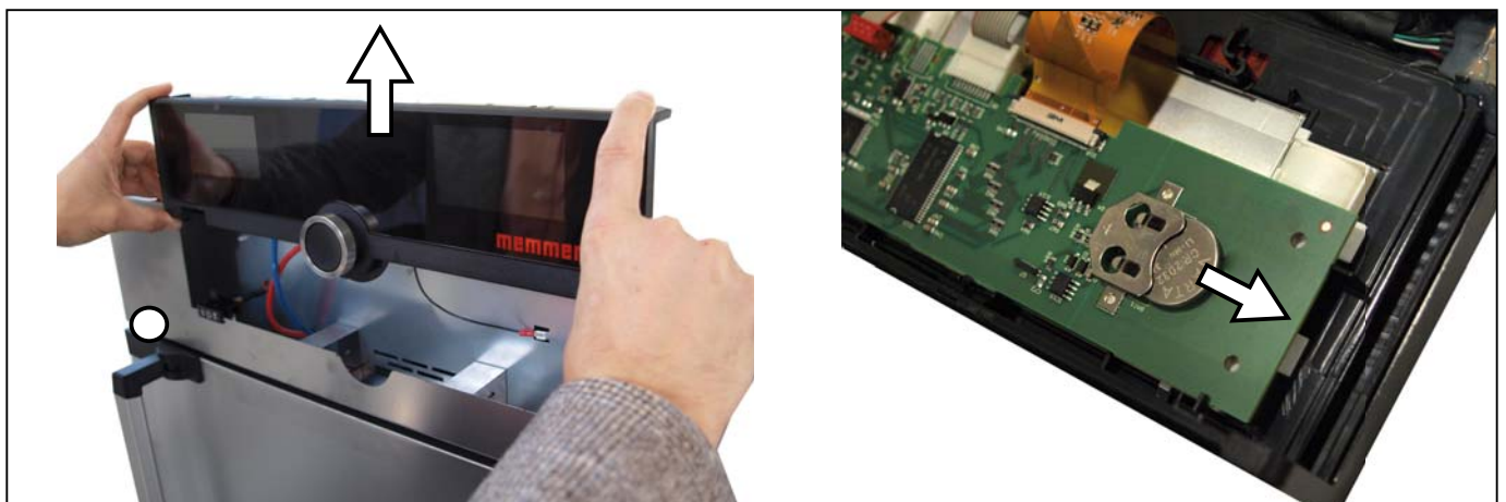
Fig. 25 Removing the lithium battery
