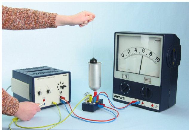
Fig. 2: Experimental set-up for the measurement of a charge that is filled into a Faraday pail by means of a hollow ball coated with graphite.
