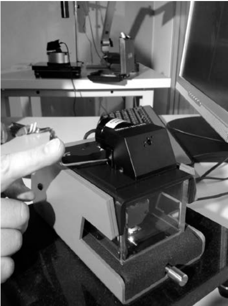
Fig. 9 Loosening of the camera sensor unit.
