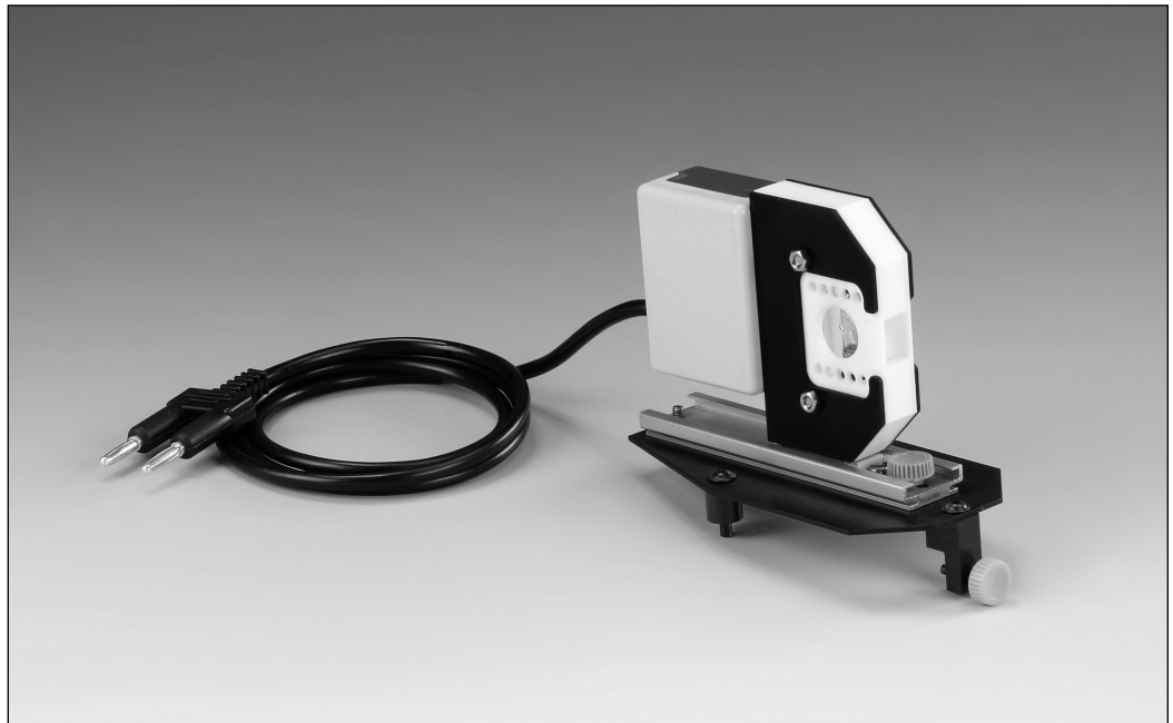
Fig. 1: Cadmium lamp for Zeeman effect 09050.20.
