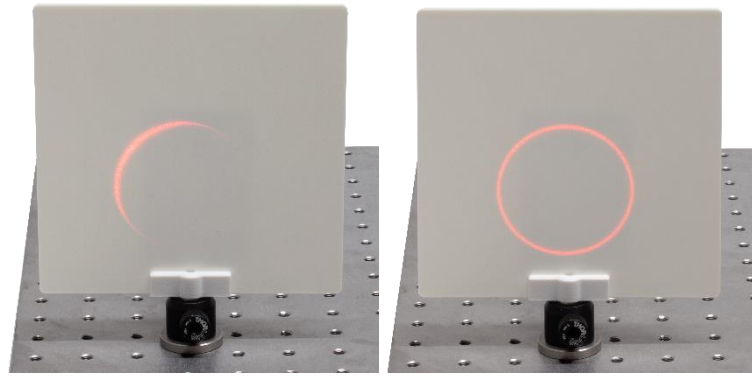
Figure 79 Axicon Pattern Before (left) and After (right) Alignment
