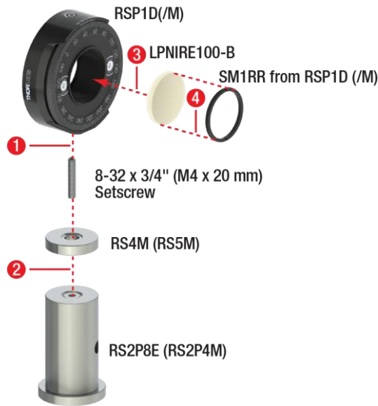
Figure 51 Large Polarizer Assembly
