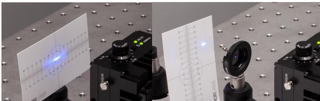
Figure 72 Beam Profile of the Pump Laser in Front of (Left) and Behind (Right) the Beam Cleaning Iris
