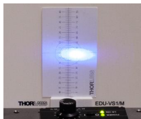
Figure 58 Laser on Screen Before Collimation
