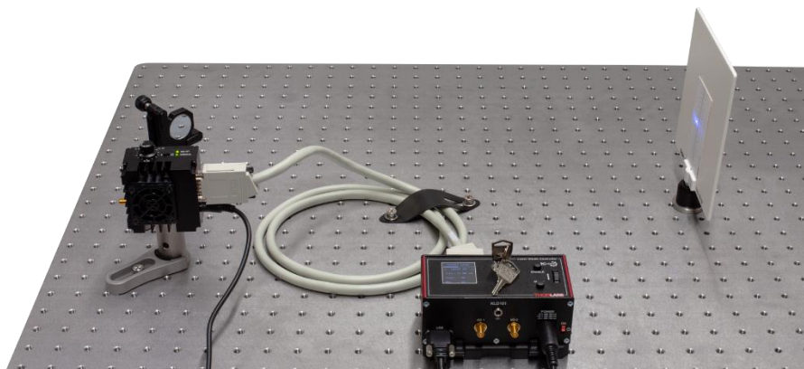
Figure 60 Collimation Setup for Compensation of Deviating Emission Angle
