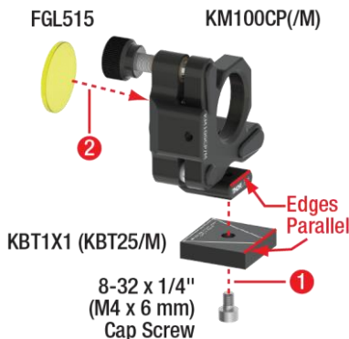
Figure 38 Glass Filter Assembly
