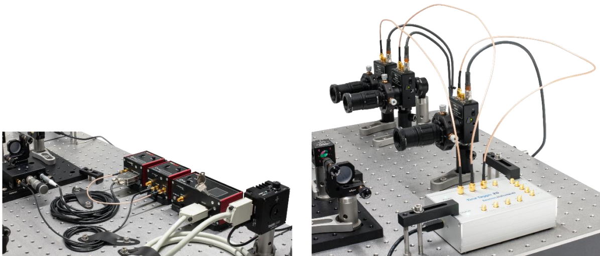
Figure 106 Cable Management for Single Photon Michelson Interferometer Setup
