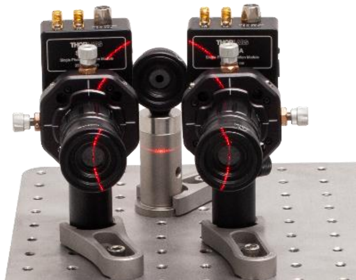
Figure 84 Detectors T (left) and A (right) after Alignment
