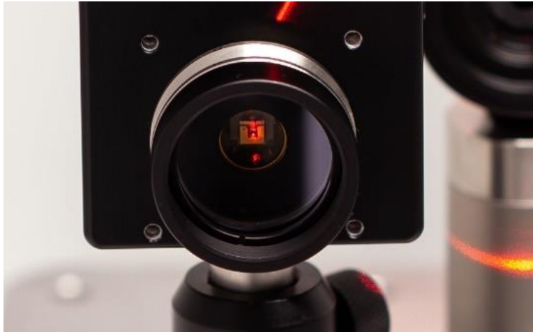
Figure 81 Laser Spot Centered on Detector Chip
