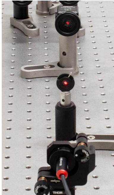
Figure 94 Additional Alignment Path After Completed Alignment (Beam Centered on Both Apertures)
