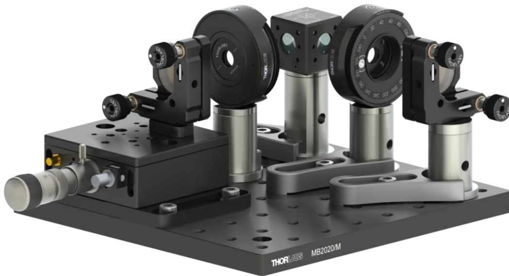
Figure 131 Orientation of the LCCs in the Michelson interferometer
