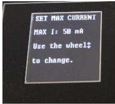
Figure 56 Maximum Current Setting for the KLD101 Controller
